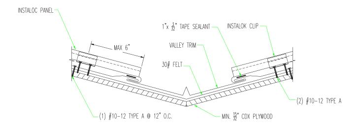
NOTE: FIELD CUT PANEL TO VALLEY ANGLE, NOTCH SEAM BACK 7/8", FOLD PANEL END INTO VALLEY HEM.
