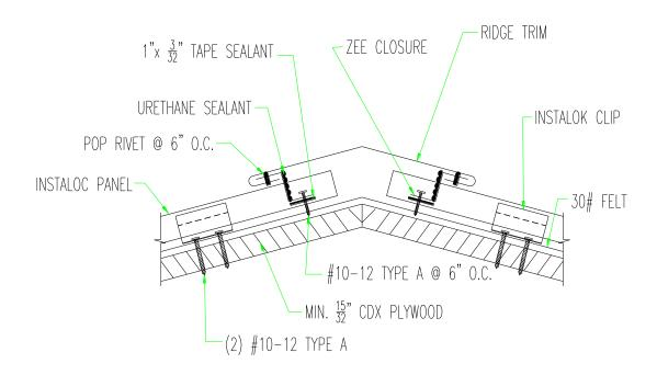
Figure 4: Instaloc Panel Ridge Detail
