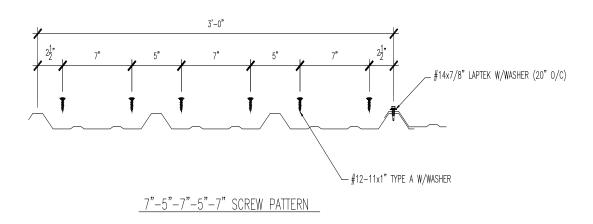
Figure 1: R, RPN, PBR Panel Fastener Attachment Pattern
