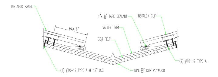
NOTE: FIELD CUT PANEL TO VALELY ANGLE, NOTCH SEAM BACK 7/8", FOLD PANEL END INTO VALLEY HEM.
