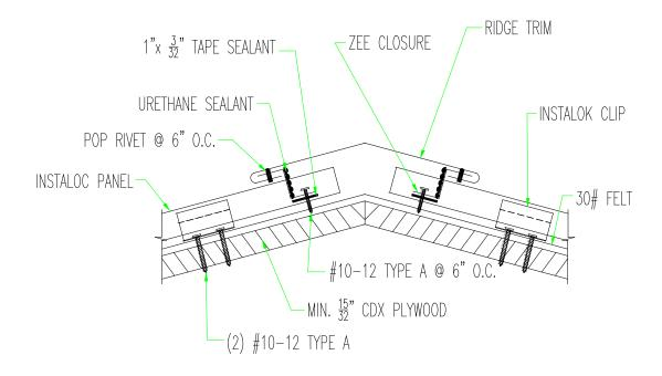
Figure 4: ABC Instaloc Panel Ridge Detail
