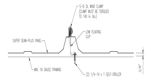
Figure 2. Super Seam Plus Metal Roof Panel with S5 DL Wind Clamps Secured to 16-gauge steel purlins (Table 2)
