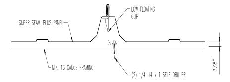
Figure 1. Super Seam Plus Metal Roof Panel Secured to 16-gauge steel purlins (Table 1)
