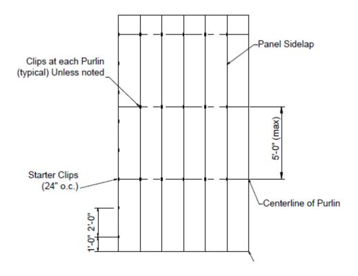
Figure 1. Minimum 24 Gauge Panel Craft 216 Panel Fastener Pattern
