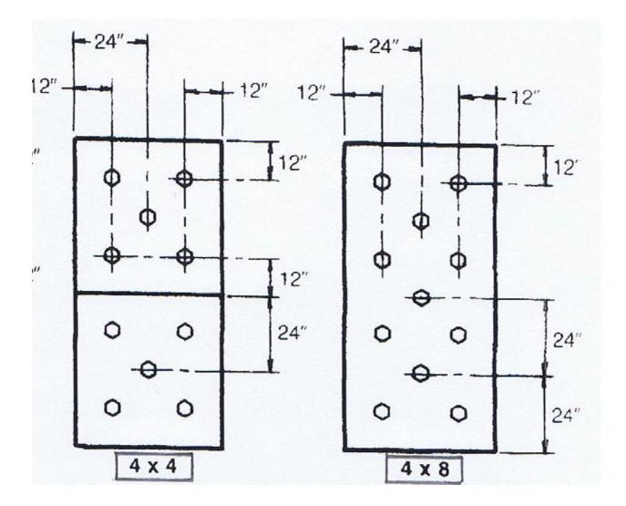
Figure 1. Insulation Fastening Patterns
