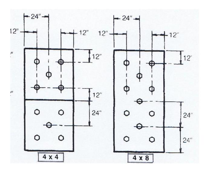
Figure 1. Insulation Fastening Patterns
