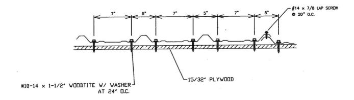
Figure 1. Fasteners at Panel Ends
