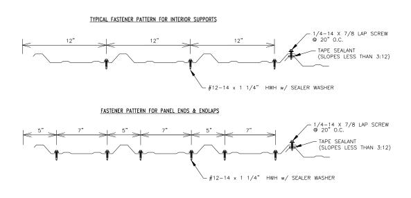
Figure 1: Minimum 26-gauge PBR Steel Panel Fastener Patterns
