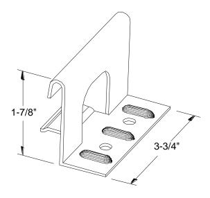
Figure 1. DMC 175S Standing Seam Panel Profile and Snap Lock Fixed Clip
