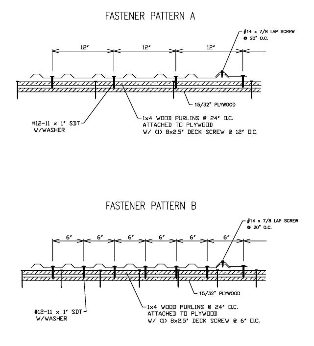
Figure 1. Fastener Pattern A and Fastener Pattern B
