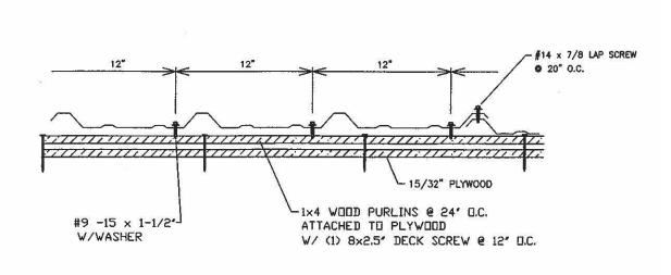
Figure 1. PBR Panel Detail (12-12-12 Fastener Pattern)
