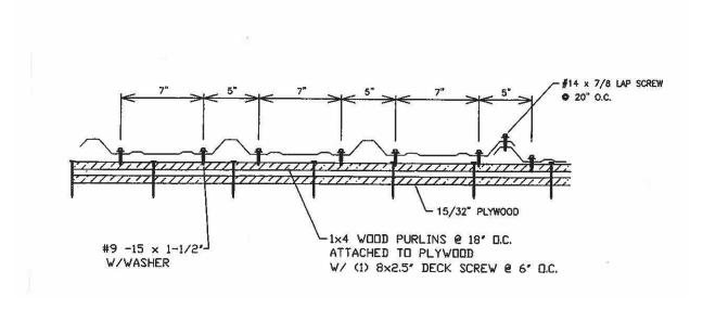
Figure 2. PBR Panel Detail (7-5-7-5-7 Fastener Pattern)
