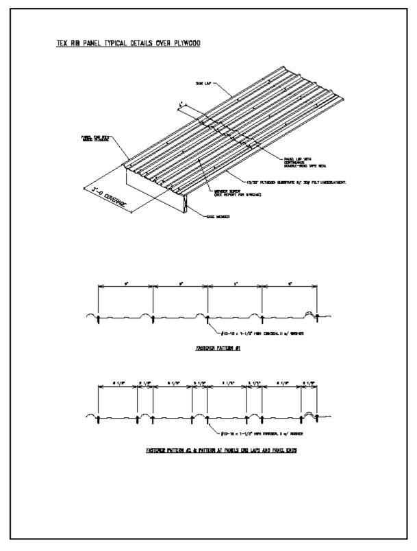
Figure 1. Tex Rib Panel Secured to Minimum 15/32" Plywood
