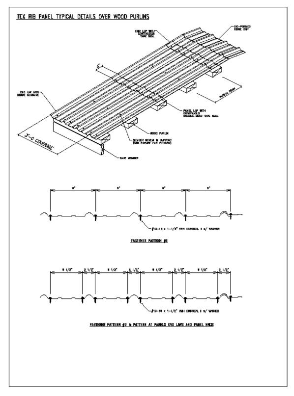
Figure 2. Tex Rib Panel Secured to Wood Purlins
