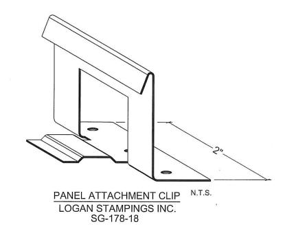
Figure 2. Tech Snap 1750 Panel Attachment Clip
