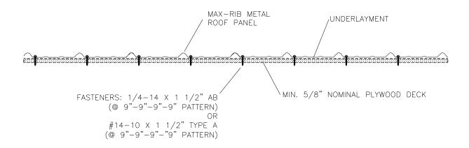
Figure 1. Max-Rib Panel Detail (Minimum 29-Gauge)
