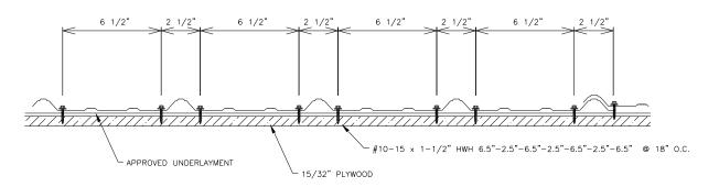
Figure 1: Sturdi-Rib X Metal Roofing Panel Secured to a 15/32" Plywood Deck
