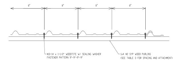
Figure 3: Sturdi-Rib X Metal Roofing Panel Secured to 1x4 Wood Purlins
