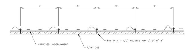
Figure 2: Sturdi-Rib X Metal Roofing Panel Secured to a 7/16" OSB Deck
