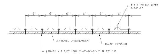
Figure 1: Low Rib X Metal Roofing Panel Secured to a 15/32" Plywood Deck
