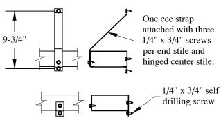
Cee strut attached to section
