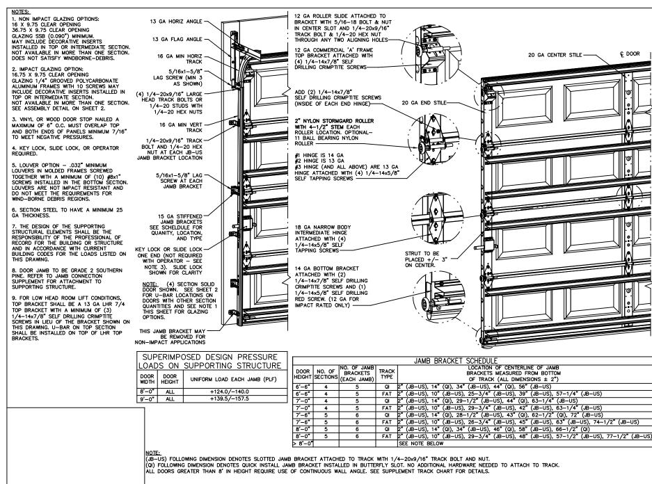
STATIC PRESSURE RATINGS APPROVED SIZES SCALE: N.T.S. SIZE: DESIGN (PSF): +31.00/-35.00 MAX WIDTH: 9'-0" DATE NAME TEST (PSF): +46.50/-52.50 MAX HEIGHT: 14'-0" 3/9/18 **ESC** IMPACT/CYCLIC RATED (YES/NO): YES MAX SECTION HEIGHT: 21" CHECKED DJK SHEET 1 OF MODELS 8000/8100/8200 DRAWING PART NO. REV. WINDLOAD SPECIFICATION OPTION CODE 1105 362403 P1
