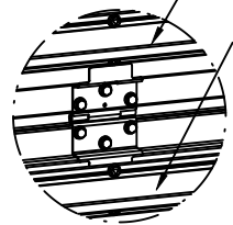
AFTER U-BAR INSTALLATION
