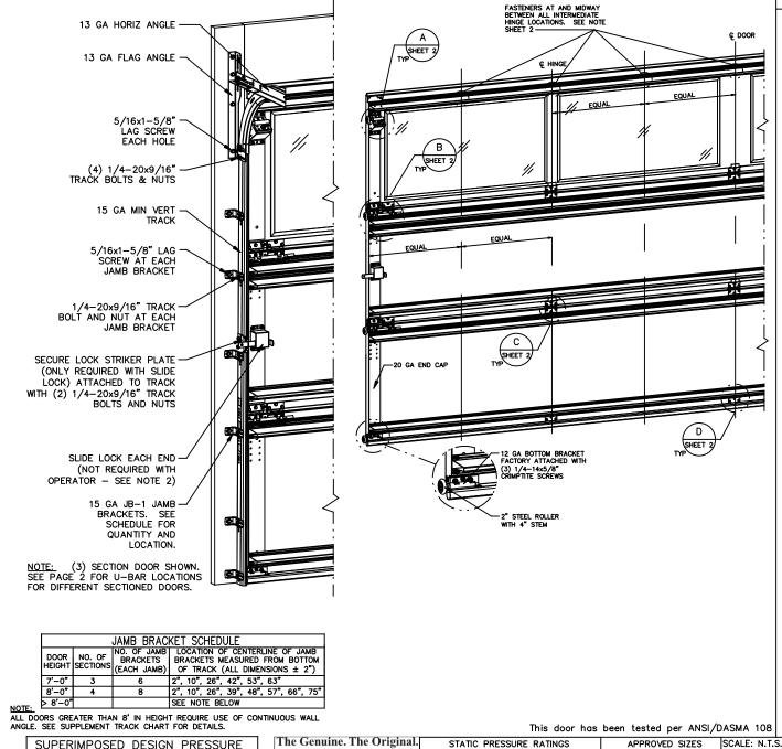
JOHN E. SCATES, PE 3121 FAIRGATE DR. CARROLLTON, TX 75007 FL PE 51737 TX PE 56308/F-2203 LOADS ON SUPPORTING STRUCTURE DOOR DOOR UNIFORM LOAD EACH JAMB (PLF) WIDTH HEIGHT +137.7/-153.0 7'-0' +137.7/-153.0 8'-0'
