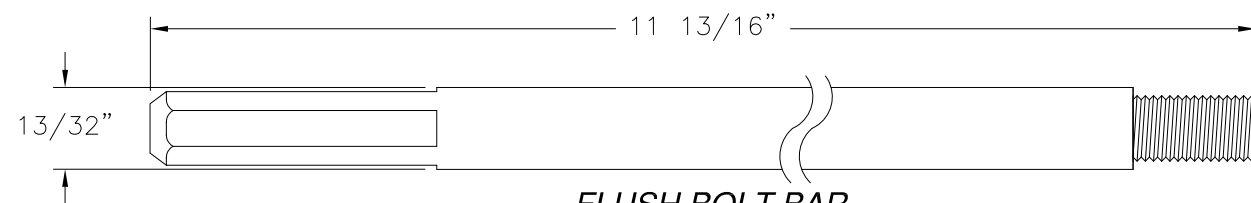
FLUSH BOLT BAR STAINLESS STEEL (SS93B) BY JAM YUAN ENTERPRISES CO., LTD
