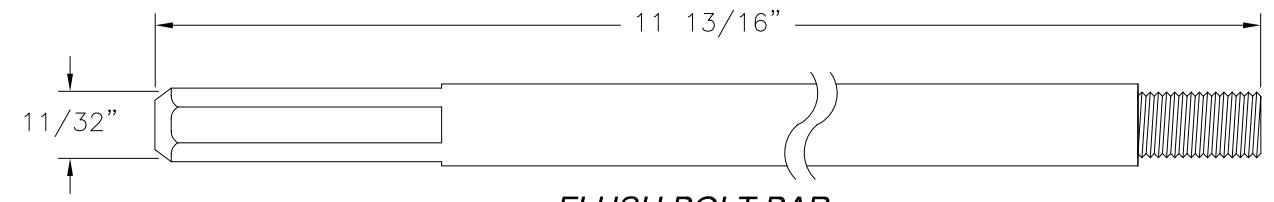
FLUSH BOLT BAR STAINLESS STEEL (SS93B) BY JAM YUAN ENTERPRISES CO., LTD
