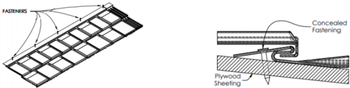
Figure 4: Direct to Deck Field Installation
