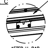
AFTER U-BAR INSTALLATION
