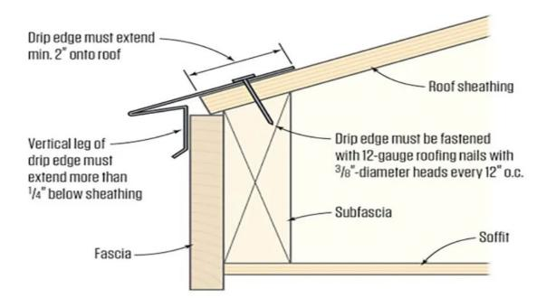
The IRC requires the drip edge to be fastened to the roof deck. The roof underlayment must be installed over the drip edge along the eaves and under the drip edge at the rake edges of the roof.
