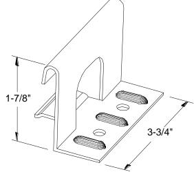
Figure 1. DMC 175S Standing Seam Panel Profile and Snap Lock Fixed Clip
