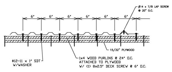
Figure 1. Fastener Pattern A and Fastener Pattern B
