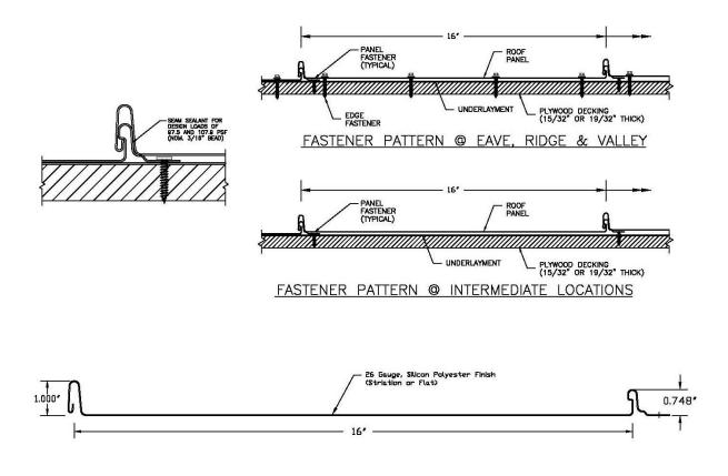
Figure 1. Advantage-Lok II Panel Detail (Minimum 26-Gauge)
