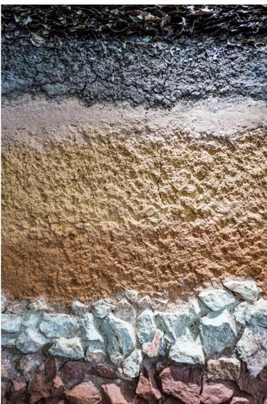
Horizontal and vertical forces within the earth keep undisturbed soil in place. An excavation disturbs or removes these forces. Soil naturally moves downward and inward due to a variety of factors, such as soil type, moisture, vibration, and surface loading.
